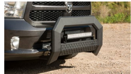
Crossbar without LEDs can be flipped to mount LED lights (see page 92 for lights)
