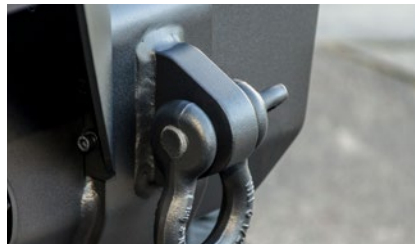
Shackle mounts accept pins up to 7/8" in diameter (#2166071 recommended)
