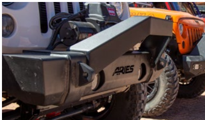
The optional angular brush guard protects the winch and front end from impacts
