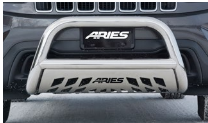
Removable, brushed 304 stainless steel skid plate deflects small road debris
