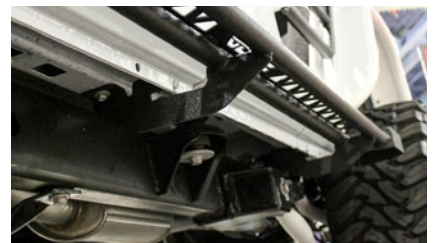
Pre-welded mounting brackets for increased strength and easy installation
