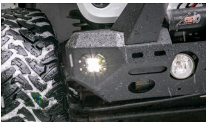
Cutouts and mounting tabs for OE lights and aftermarket LEDs (see page 92 for LED work lights and light bars)
