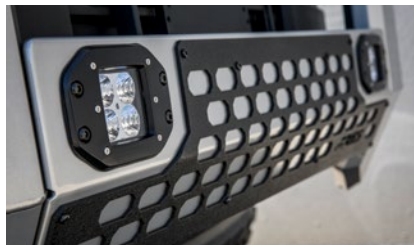
Optional flush-mount LED work lights built into the crossbar add function and style
