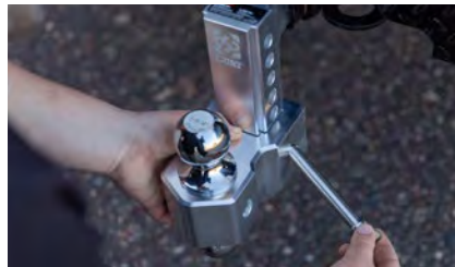
Dual ball attachment eliminates extra attachments by providing two ball sizes in one
