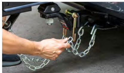
Hooks maintain proper safety chain function for trailer disconnect
