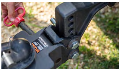
Head-tilt adjustment feature provides 15° of adjustment for precise leveling
