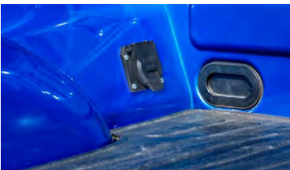
10' routes socket closer to truck cab
