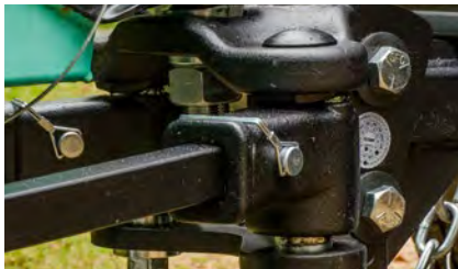
Integrated sway control actively resists sway and levels the vehicle and trailer
