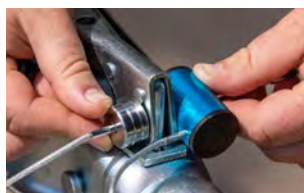
Coupler lock can also be used while towing to secure the trailer
