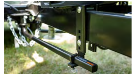
Adjustable brackets provide fixed support unlike spring bar chain models
