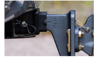
Reduces the receiver tube opening to fit smaller shank sizes
