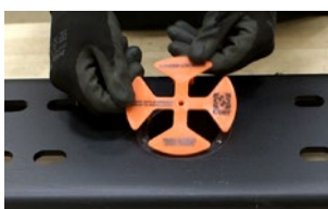
Step 1 - Place Center Locator in the gooseneck hitch ball hole
