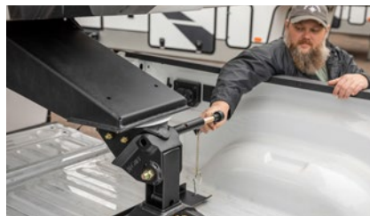
Easy-to-reach release handle for ergonomic locking and unlocking operation of the head from the side of the truck bed
