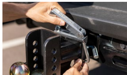
No-tool installation and easy-to-adjust clamp lever (#22325, #22320 only)
