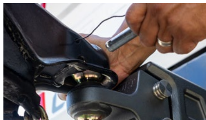
Latchless, one-pin coupling is easier to use than traditional couplers
