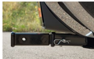
Moves coupling point farther from the vehicle to avoid obstructions
