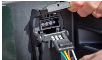
Plugs into USCAR socket to provide 4- and 7-way trailer wiring connectors
