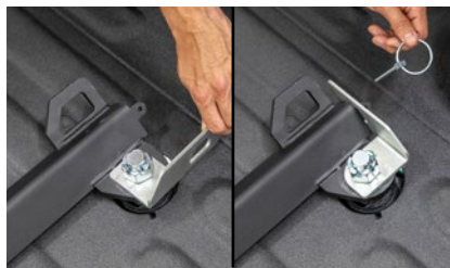
Patented quarter-turn mechanism allows for quick, easy installation
