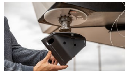
Head piece bolts onto kingpin, allowing head channel to guide the kingpin into place for easier hookup
