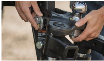
Quick, easy tilt adjustment feature simplifies setup and installation (excluding 17501)
