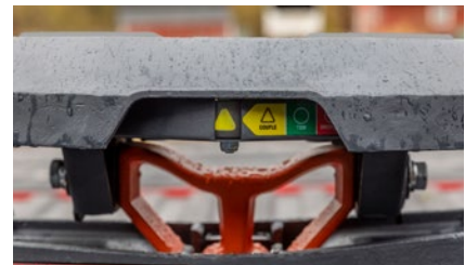
Three-position coupling indicator clearly shows coupling status
