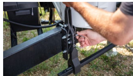
Adjustable brackets provide fixed support unlike spring bar chain models
