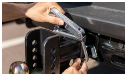
No-tool installation and easy-to-adjust clamp lever (#22325, #22320 only)
