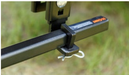
Two points of sway control use friction to distribute weight evenly, keeping trailer aligned
