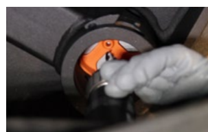
Step 3 - Use Center Locator to drill pilot hole to drill pilot hole up from under bed
