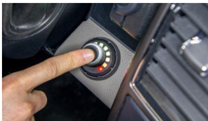
Controls manual override and all brake settings with a simple push-button rotary knob
