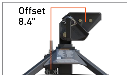
Offset 8.4" Coupling point offsets 8.4" rearward for added turning clearance (16051 / 16602 only)
