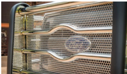
Heavy-gauge, punched steel screen provides extra grille protection from rocks and debris
