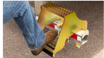
Grated steps provide exceptional traction, even when wet
