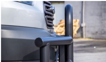
3" diameter, 14-gauge stainless steel tube design for added vehicle protection
