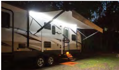
Integrated lighting track makes it easy to add the Solera LED light kit to the RV
