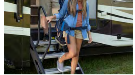
Handrail makes it easier and safer for campers to get in and out of their RVs
