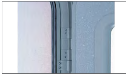
The integrated felt seal helps prevent water from infiltrating your trailer
