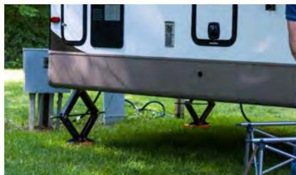
Rated to support up to a 5,000 lb. load capacity per jack
