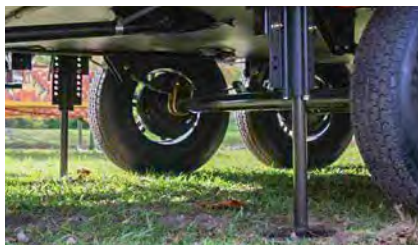
Patented aluminum leveling jacks are about 70 lbs. lighter than competing systems
