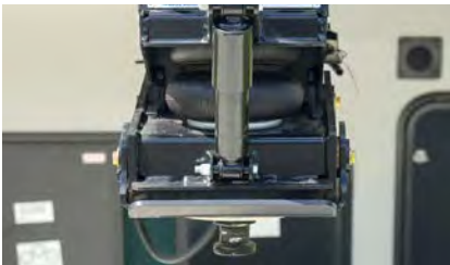
Air Ride technology combined with Rota-Flex pivoting head significantly reduce fore-to-aft movement and vertical tug-of-war
