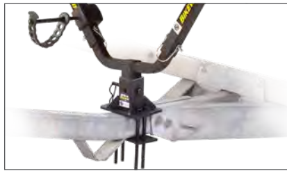
Attaches to Bump-It® for towing vehicle applications (sold separately)
