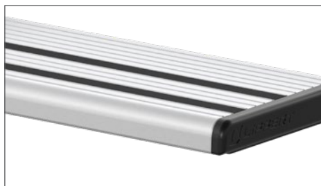
Anti-slip rubber for safe entry and exit
