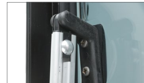
Tubular or automatic stays allow for opening in every position
