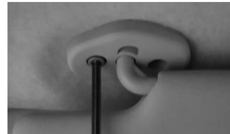
Installs under the existing sun visor pivot cover
