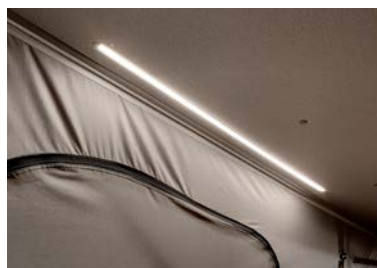
Two rooftop LED light strips provide overhead lighting
