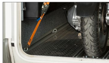
Allows bikes and motorbikes to be secured in the motorcaravan's garage
