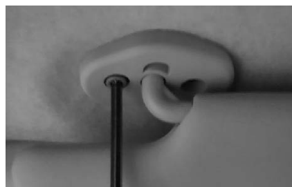
Installs under the existing sun visor pivot cover
