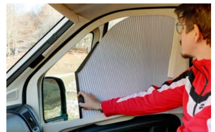
PVC and aluminum handle for manual operation
