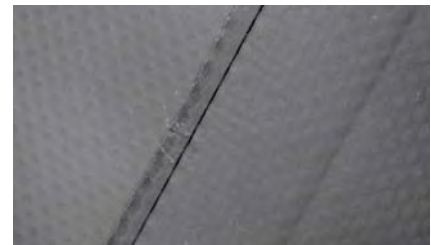
Welded seams have no glue to harden or breakdown
