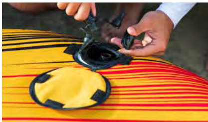
One-way boston check valve with two ports for easy inflation and quick deflation of inflatable boats
