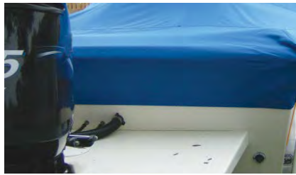
No cut out patterns for boats with sea mount style engine bracket - no cut out in stern section
