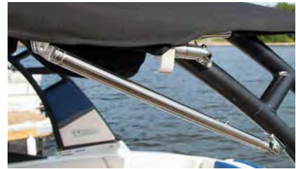
Bright-dip, anodized aluminum frame tubing uses high quality marine grade hardware
