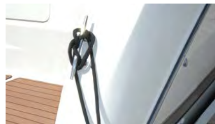
Bow and stern lines should be two-thirds the length of your boat. Spring lines should be as long as your boat
